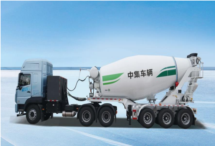
Electric tractor-trailer mixer truck (Model: J-RT1.0 mixer truck)
